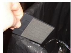
As necessary, gently tap the filter over a garbage can to loosen the dirt particles. If needed use a compressed air can to gently spray out dirt.
